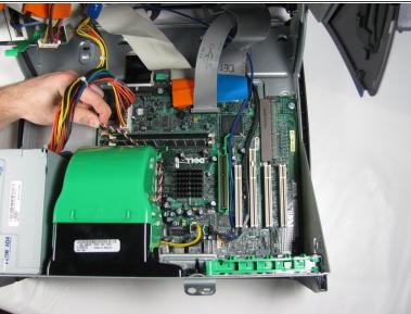
Disconnect the fan cable from the motherboard.
