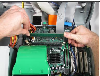
Push out on the cream colored tabs on each side of each RAM module until it pops up and out of its slot and remove the RAM.
