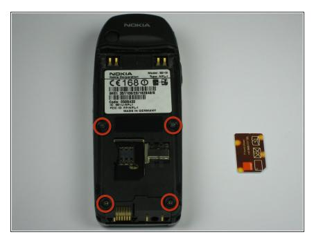
Unscrew and remove the four T6 Torx screws.
