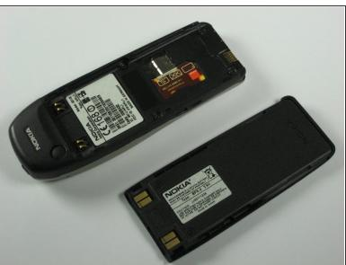
Press and hold the battery release button and slide the battery away from the Nokia logo
