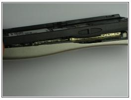
• Insert a plastic opening tool between the faceplate and the black backplate. Gently pry them apart, working from the lower end to the upper side of the phone.
