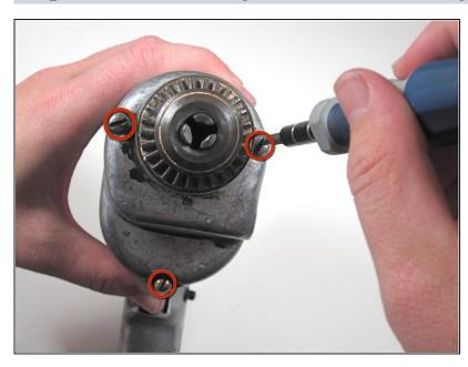
On the front of the drill, remove the three 2" flathead screws connecting the front housing to the rear housing.
