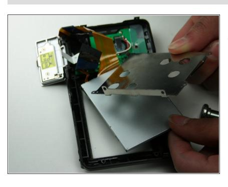
Lift out and remove the metal plating over the LCD screen.
