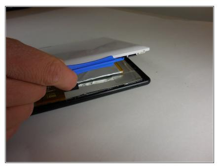
Remove the back casing by slowly popping each tab out with a plastic opening tool.
