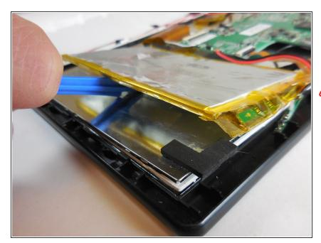
• To remove the battery use an iFixit opening tool to pry the battery apart from the sticky glue.
