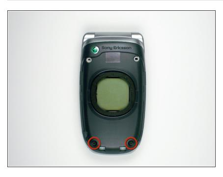
To remove the front grey case, remove the two screws shown with a T5 Torx Screwdriver.
