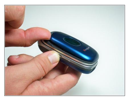
To remove the front cover, lift up the case with a fingernail in the small slot as shown.
