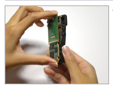
• Lift the logic board out of the phone.
