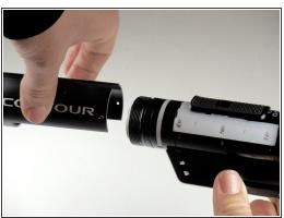
Grab the camera on both sides and slide the outer shell forward until completely removed.
