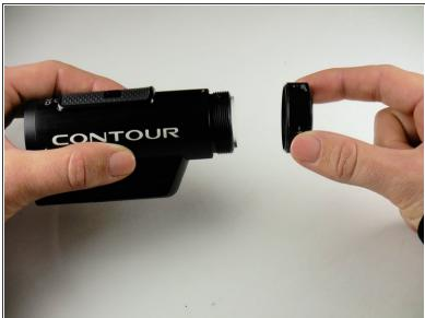
Rotate the metal ring counterclockwise until completely removed.
