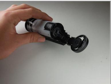
Open the back door by your thumb and index finger on sides of back door and pull upward.
