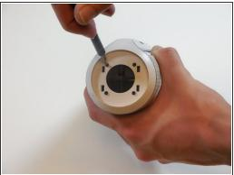
Unscrew four 3.3mm screws on each end of the JBL using a size 1 ph screw driver (8 screws total).
