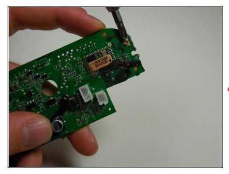
Use the soldering iron to desolder the U.FL antenna connector. You might need to use a desoldering braid wire to remove the excess of solder.
