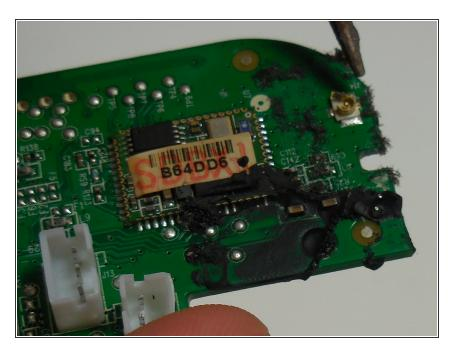
Locate the underside of the motherboard, where the square U.FL antenna connector is.
