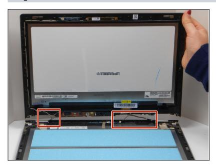
• Detach the screen from the front panel by sliding the screen up about 2mm. Do not pull too far, as there are still connected wires.
