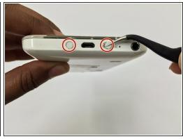
Lastly, reinsert the screws at the bottom of the device, as well as the screw beside the SD Memory Card port.
