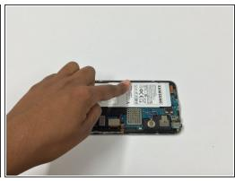
Insert the new battery into its position, and reconnect its tab onto the motherboard.
