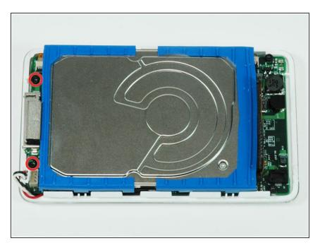
Remove the 2 black T6 Torx screws from the left side of the logic board.
