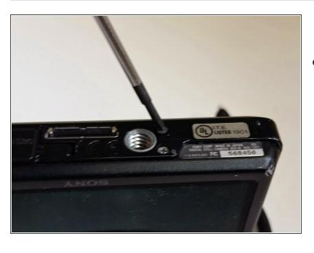
Use the Phillips #00 screwdriver to remove the 4mm length screws.
