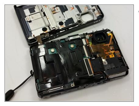
This is the camera with the front cover unscrewed and partially removed.
