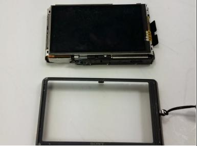
Remove the back cover so that the back cover is now completely separate from the body of the device. To reassemble your device, follow these instructions in reverse order.
