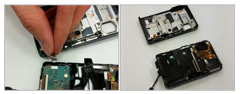
Pull the ribbon out of the connection port so that they are completely disconnected.
