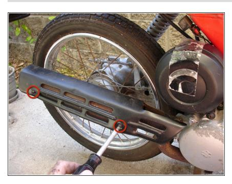
Use a #2 Phillips screwdriver to remove the heat shield from the muffler.
