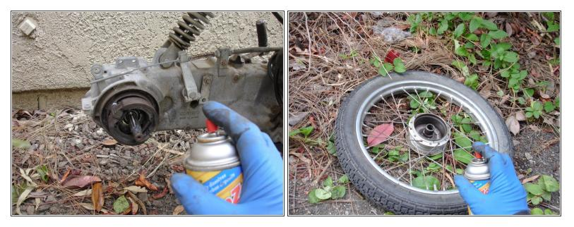
Thoroughly spray the the brake shoe assembly and inside of the brake drum with a brake cleaning solvent.
