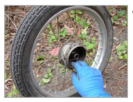
Once the solvent has had a chance to work its magic (10 minutes or so), use a rough-grit sandpaper (100 grit or so) to clean the inner diameter of the drum. Rinse and repeat until you are satisfied with the cleanliness of the drum.
