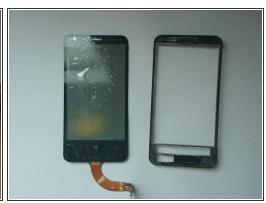
Continue with the separation by using a plastic tool.
