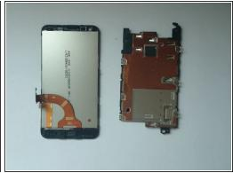
The Midle frame is held by 6x locking clips, three on each side. Release them and remove the Middle frame.
