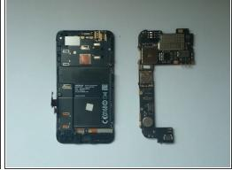
With a plastic tool gently release the mother board and remove it.
