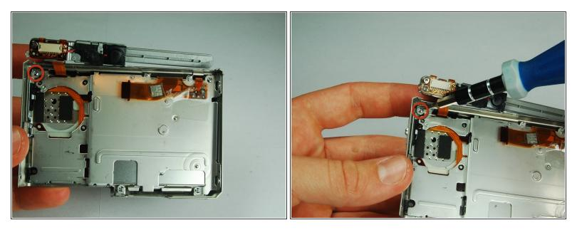
Use a PH00 screwdriver to remove the 2.9 mm phillips screw on the upper left side of the case.
