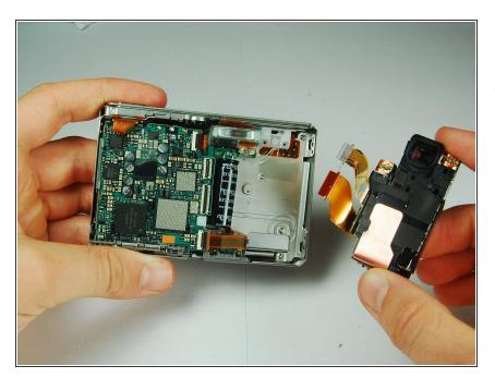
Grasp the CCD Sensor Module and remove it.
