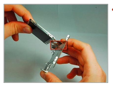
Pull the tape off that holds the LCD to the assembly.
