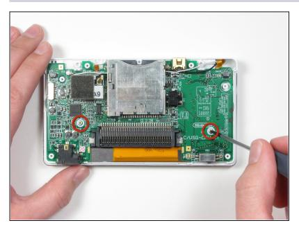
After taking the bottom case off, remove two Phillips #00 screws that secure the logic board to the plastic case.
