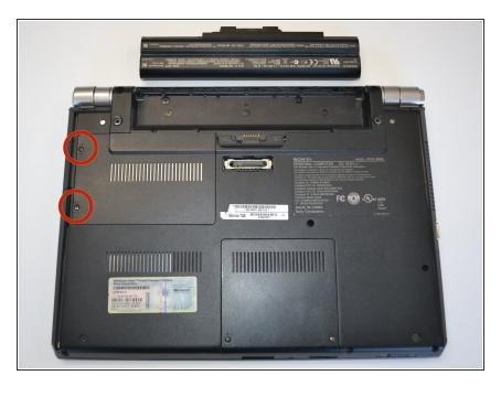
Using a Phillips #1 screw driver, loosen both screws holding the cover in place. These screws are secured to the cover with retaining clips.
