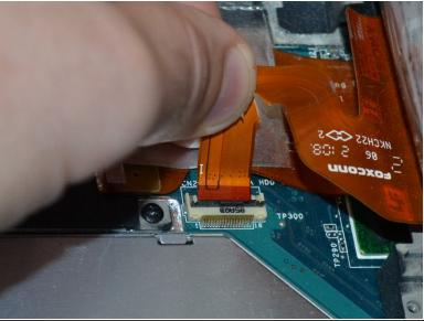
Grasp the ribbon cable carefully near the connector end. Remove it by pulling the cable away from the connector on the motherboard at a slightly upward angle. To reassemble your device, follow these instructions in reverse order.
