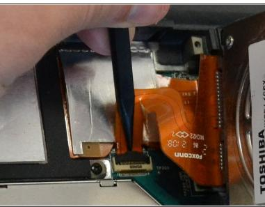
Use the spudger or a fingernail to carefully release the lock securing the ribbon cable to the motherboard.
