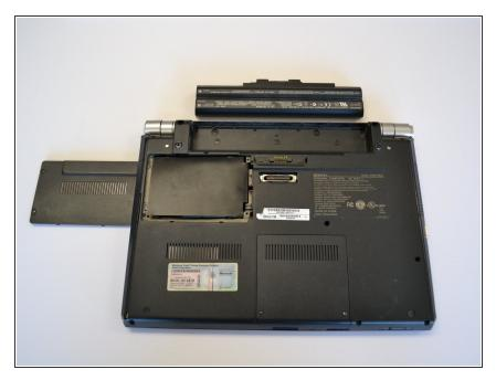
Lift the cover with a fingernail or plastic opening tool from the side where the screws are present and lift it off to the left.
