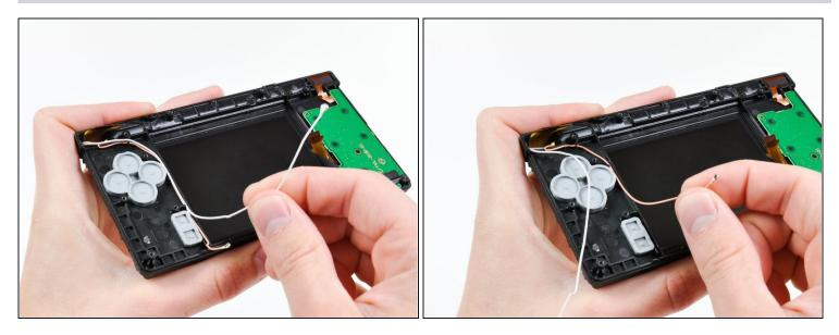
• Continue de-routing the microphone and Wi-Fi antenna cables through the opening located on the bottom DSi's framework.
