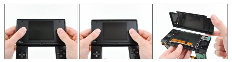
• Using two hands, gently slide the rear bezel upwards.
