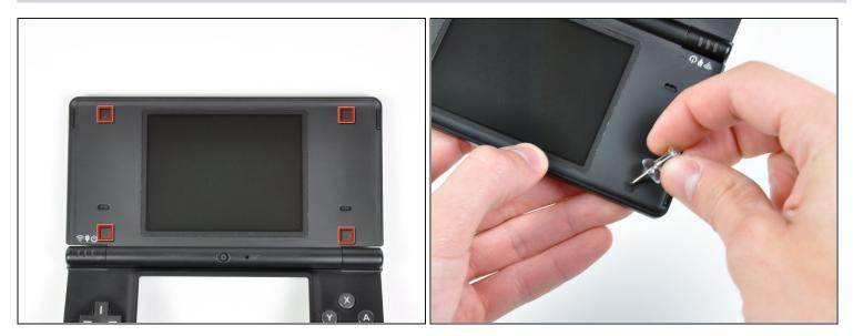
• Use a pushpin to remove the four plastic screw covers on the front bezel.
