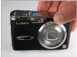
• Carefully remove the upper assembly, which houses the buttons and the flash battery.
