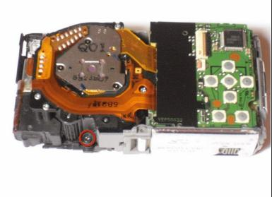
Remove the three black 5mm screws attached to the lens frame.
