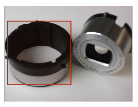
Remove the first lens frame from the lens assembly.
