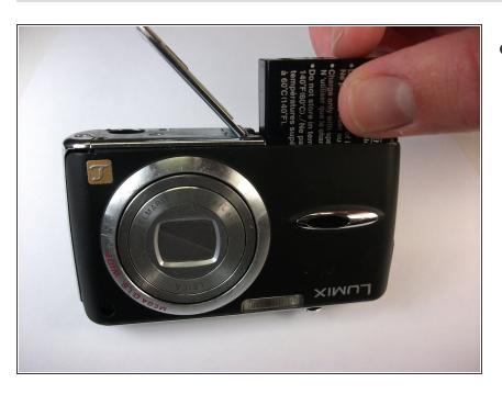
Remove the battery from the camera.
