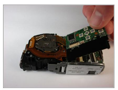
Lift out the circuit board as shown.
