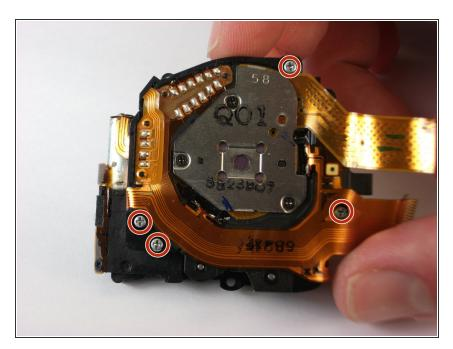
Remove four 4 mm screws from the lens assembly using the Phillips #00 screwdriver.
