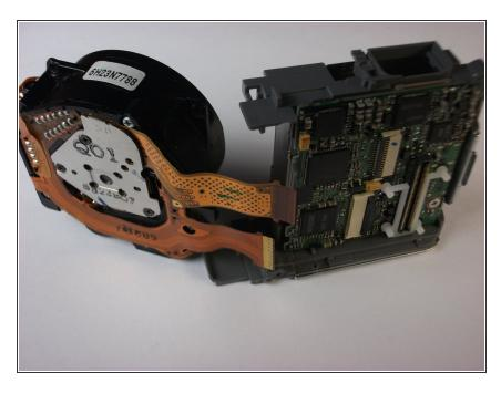
Remove the lens assembly as shown.
