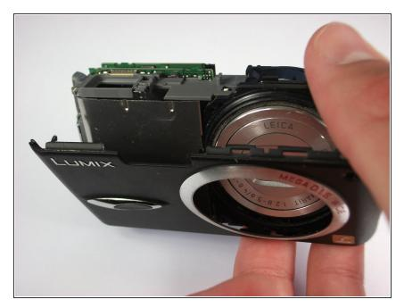
Carefully remove the front casing after verifying that the thin plastic around the lens is not still attached.
