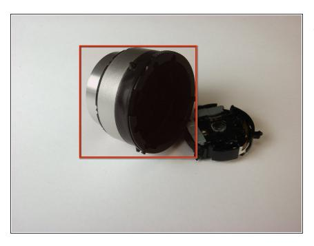
Detach the second frame unit from the lens assembly.
