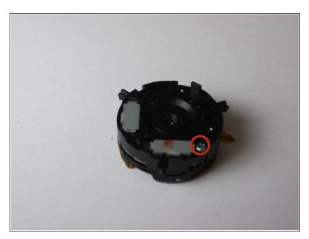
Remove the 4m m screw from the lens housing using the Phillips #00 screwdriver.
