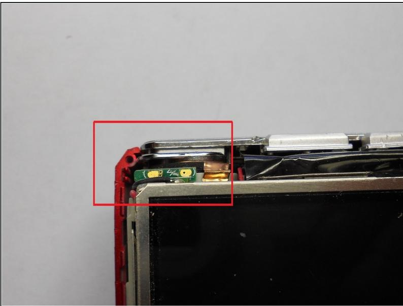
⚠ This is where energy for the flash is stored. Even with batteries removed, if you touch these connections, you can be shocked, depending on if the flash capacitor has a stored charge. It may not have a stored charge, but work around this assuming it does.
