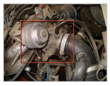
Locate throttle body on right side of engine, it is between the intake tube and intake manifold.
