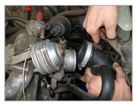
Remove the intake tube from the throttle body.
