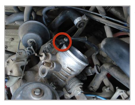
Locate wiring clip on the underside of the throttle body.
