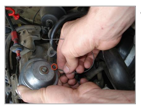
Slide both slackened cables off assembly's guides.
