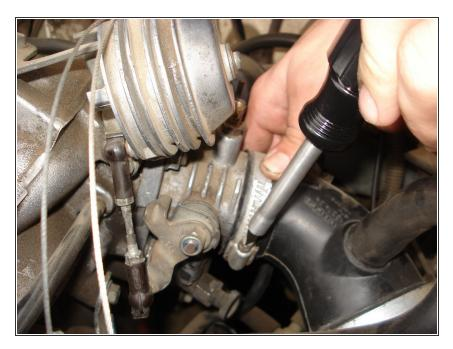
Use a flat head screwdriver to loosen the hose clamp attaching the intake tube to the throttle body.
