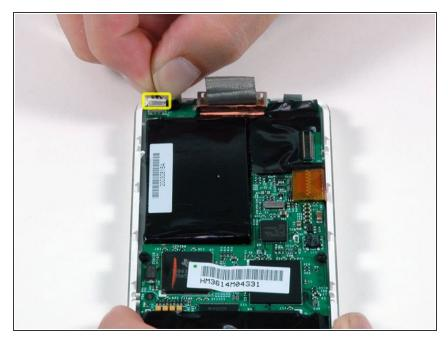
Carefully disconnect the white battery connector from the logic board. Be sure to pull only on the connector itself and not on the cables.
