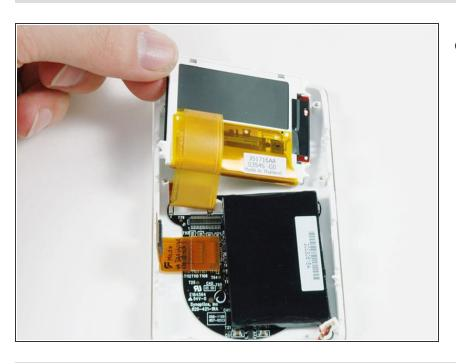
Lift the display panel out of the iPod.
