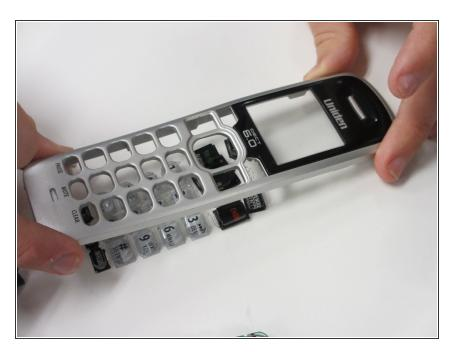
Remove plastic buttons from outer shell.
