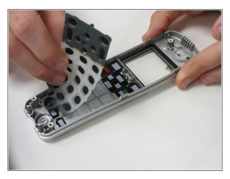
Remove the rubber keyboard layer.
