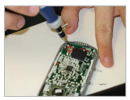
Remove screw (4mm head,8.6mm length) from circuit board.
