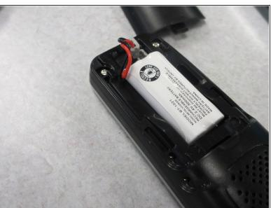
Slide the battery cover off of the handset, and unplug the battery.
