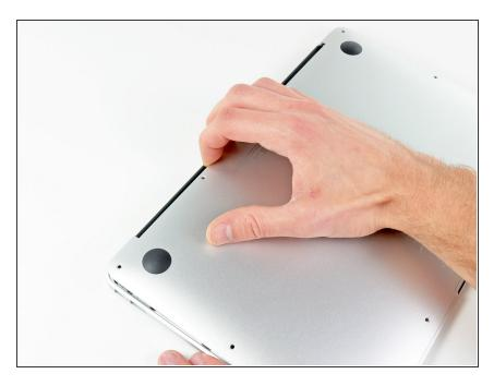
Wedge your fingers between the display and the lower case and pull upward to pop the lower case off the Air.
