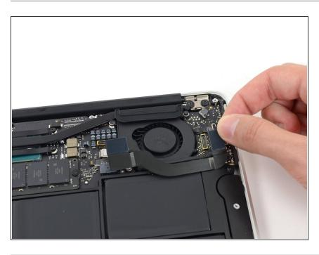
Lift and remove the I/O board cable.
