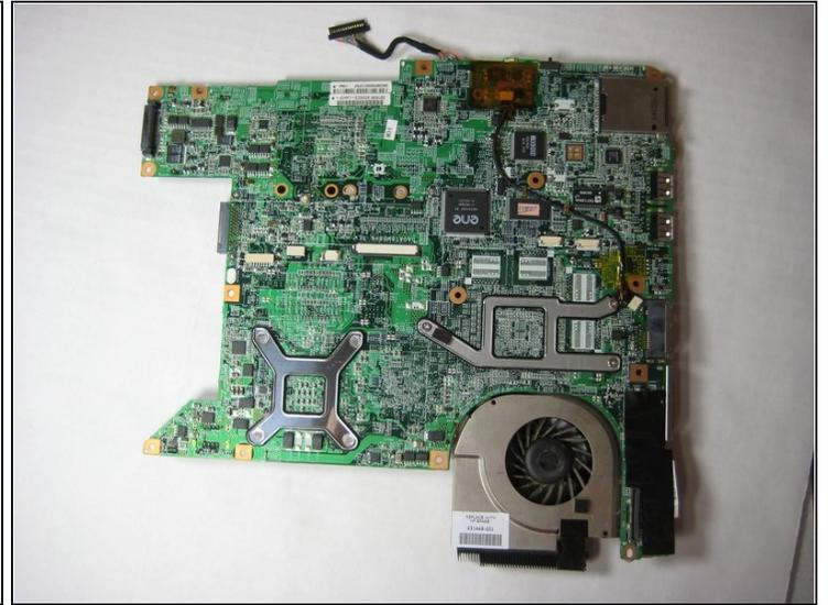
☑ Carefully set the motherboard on a non-conductive and level surface.
