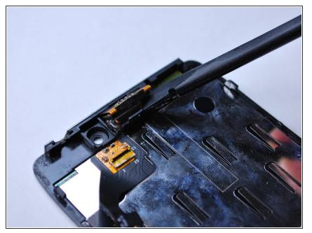
Insert the spudger between the speaker and retaining clip and gently pry upward to release the earpiece speaker.
