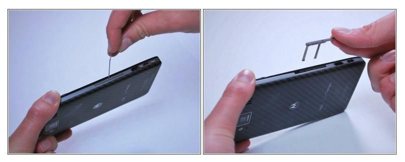
To remove the SIM card, use an unfolded paperclip to press down on the metal plate on the left side of the phone until it pops up.
