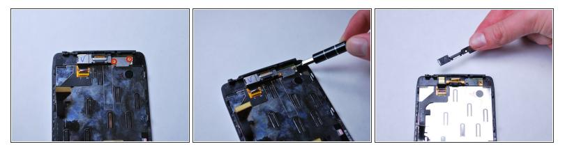
With a Torx T3 screwdriver, unscrew the two 2.0 mm screws on front-facing camera mounting bracket. Then lift to remove it.
