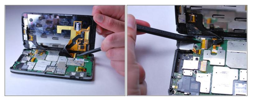
Release the two black ribbon flex cables by gently pulling up on the connection using the spudger.
