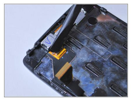
On the back of the LCD display, release the yellow front-facing camera ribbon cable by gently lifting upward on the black retaining clip with the spudger.
