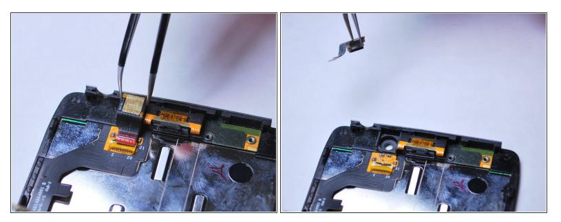
• Use tweezers to remove the front-facing camera by lifting it from the LCD display frame.
