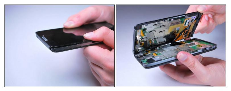
• Gently push the screen toward the top edge of the phone and tilt the screen to reveal the black flex cables.
