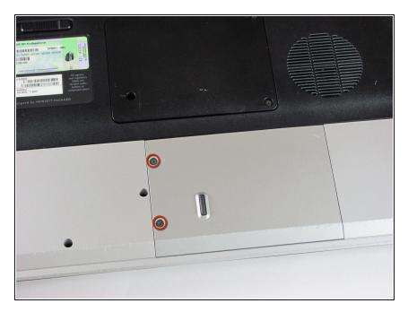
• Remove the two screws securing the hard drive cover.
