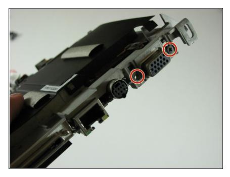
Remove the two 10.0 mm screws securing the fan on either side of the external monitor port.
