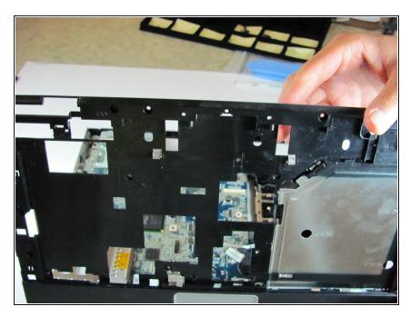
• Lift the top cover off of the rest of the computer frame.
