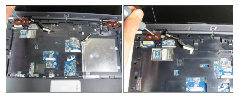
• Remove the four 7.0mm screws securing the screen to the computer.
