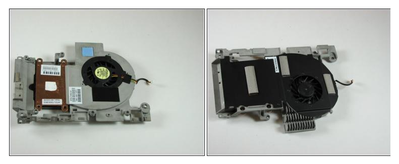
• Remove the fan from the computer frame.
