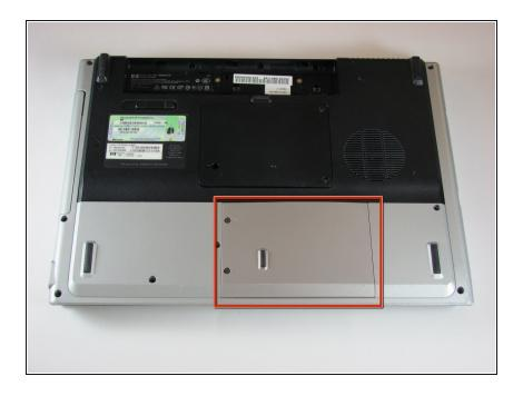
• Locate the hard drive cover. Note that in this image, the RAM cover is still in place.
