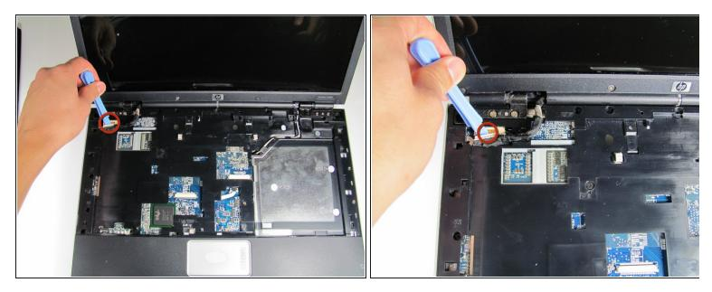
• Use the plastic prying tool to disconnect the screen cable from the system board.
