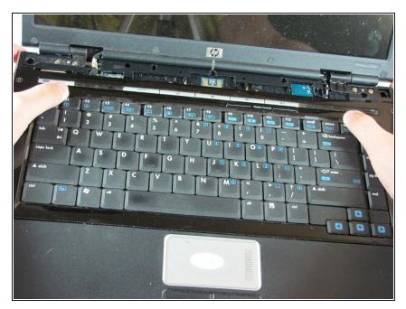
Next, remove the keyboard. Push on the keyboard frame above the function keys and slide the keyboard toward the screen.
