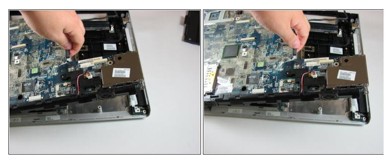
• Lift the system board off the computer frame.
