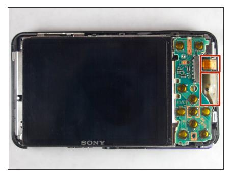
These are the two cables connecting the LCD screen to the motherboard below the screen.
