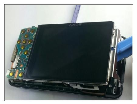
Remove the LCD screen from the side opppsite the battery terminals.
