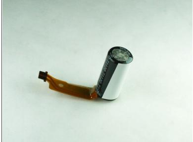
After camera is disassembled the capacitor will need to be removed. Use tweezers to gently pull away the ribbon from the connector.
