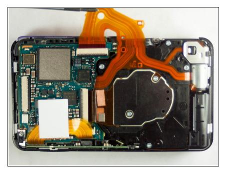
This is what the camera should look like after 2 cords and the screen have been removed. The lens cord is being held to the side for a clearer view.
