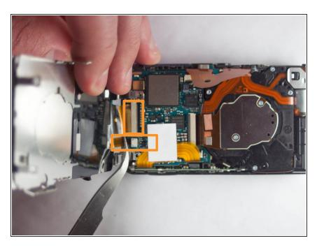
• Pull these two cords straight back to disconnect them from the respective housings. Caution: The housing do not need to be moved or adjusted in anyway. Do not pull the cords at an angle, it can destroy the cords and the housing. Pull Straight Back!
