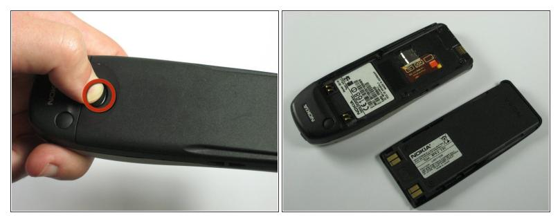
• Press and hold the battery release button and slide the battery away from the Nokia logo
