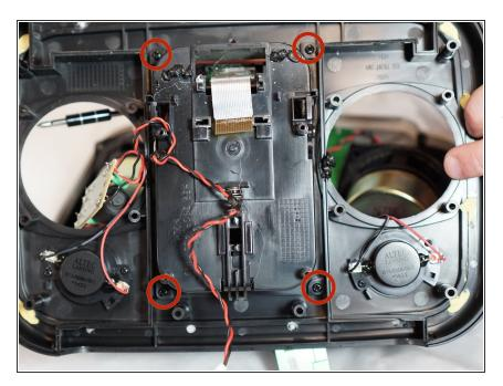
To remove the iPod Dock, unscrew the four 8mm screws located on the corners of the dock casing using the Phillips #1 screwdriver.
