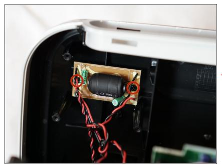
Repeat the previous step on the other side of the speaker. There are two more 7mm screws on the filter mirroring the first.
