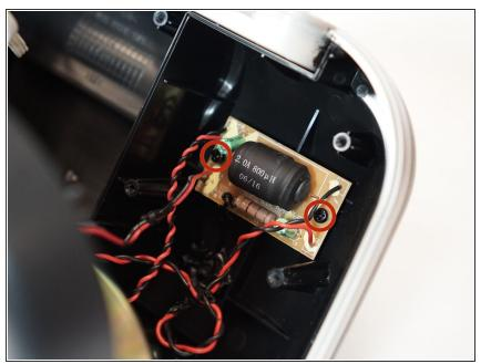
Using a Phillips #1 screwdriver, remove the two 7mm screws from the filter.
