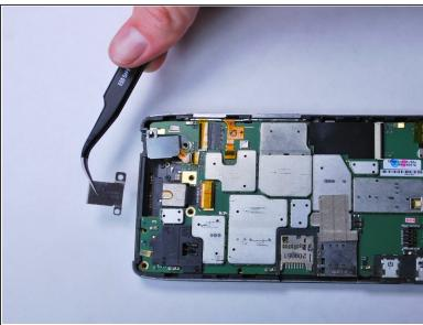
Using tweezers, remove the back facing camera cover.
