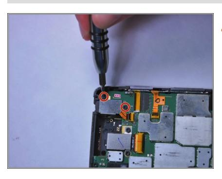
Use the Torx T5 screwdriver to remove two 4.0 mm screws on the cover of the headphone jack in the upper right corner.
