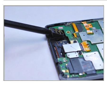
Using the pointy end of the spudger, gently pry the headphone jack from the motherboard and remove it. To reassemble your device, follow these instructions in reverse order.
