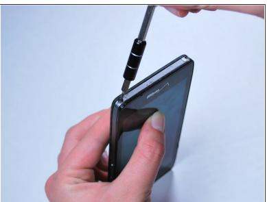
Use the Torx T5 Screwdriver to remove two 5.0 mm screws at the bottom of the phone.
