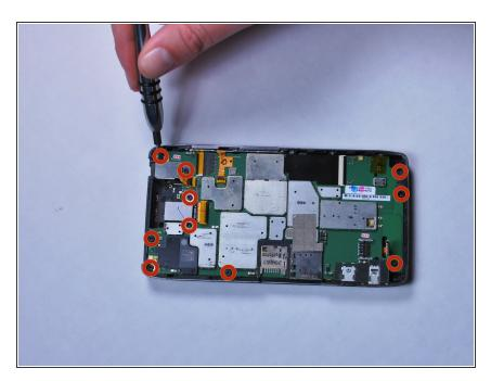
Unscrew all ten 4.0 mm screws on the motherboard using a T5 Torx screwdriver.
