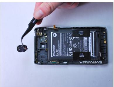
Use tweezers to remove the speaker from the top left of the phone by pulling upward.
