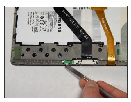
Use the flat end of the heavy-duty spudger to lift the white microphone piece until it is removed from its socket.
