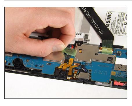
Using your fingers, remove the green tape covering the battery connector.
