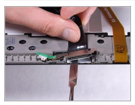
Lift the charger port with the flat end of the heavy-duty spudger and remove it from the device.
