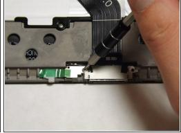
Use the Phillips 000 screwdriver to unscrew the two 3mm screws holding the charger port in place.
