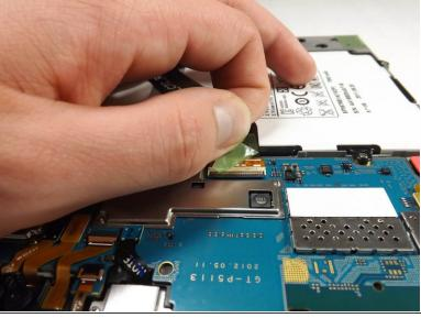
The charging port cable is the black cable connected to the charger port. Using your fingers, peel the green tape off of the charging port cable connector.
