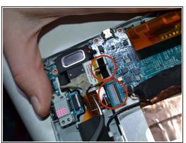
Continue to disconnect all resistors attached from the motherboard, using tweezers.
