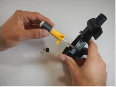
Hold the impeller cover with one hand and the impeller with the other. Slide the impeller out.
