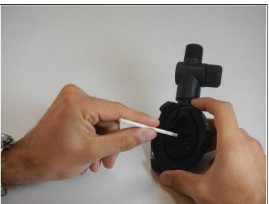
Hold the impeller spindle and wiggle it side to side until it detaches from the impeller cover.
