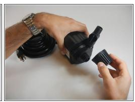
Hold the inlet screen and rotate it counterclockwise to unscrew it. It is helpful to remove the inlet screen so that it is not damaged during the replacement process.
