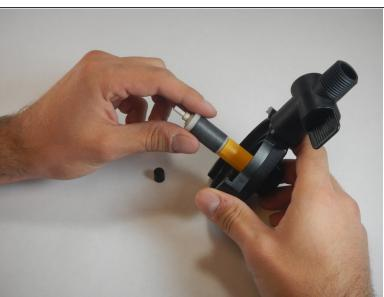
Remove the rubber stop that is attached to the tube that runs through the middle of the impeller.
