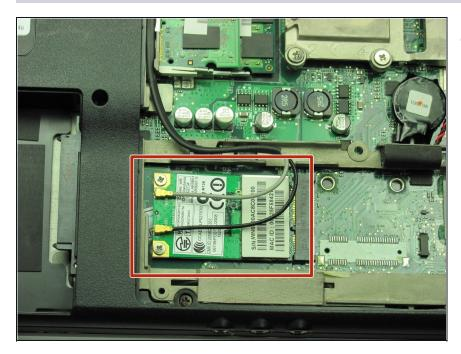
*i* The wireless card is located to the right of the hard drive and below the RAM.
