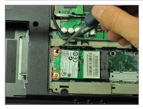
• Remove the two screws next to the wires with a Phillips #00 screwdriver.
