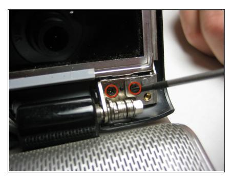
Hold on to the LCD screen to prevent it from falling over and remove the two 3.58mm screws on the sides at the bottom.
