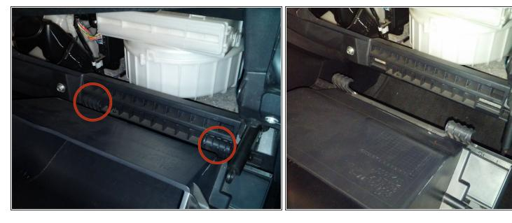
• The glove compartment can now be removed completely by raising it off its hinges.
