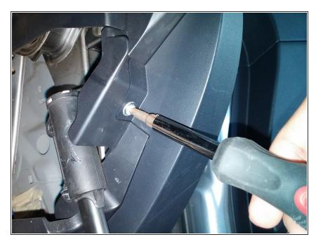
Using the Philips #2 screwdriver, remove a 15 mm screw located just above the glove compartment damper piston.
