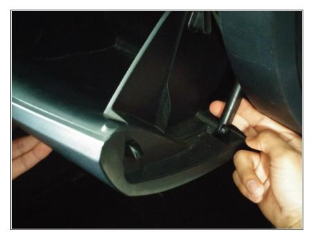
Remove the attached plastic arm by simply pulling outward so that the arm snaps out of its socket.
