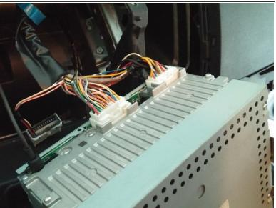
Pull out the radio unit to expose the connections behind it.
