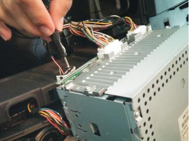
Remove the black antenna connection by simply pulling it out.
