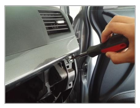
Using a Philips #2 screwdriver remove a 15 mm screw from the trim piece.
