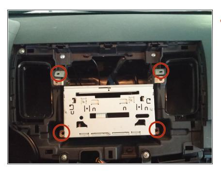
Using a Philips #2 screwdriver remove four 12 mm screws attached to the mounting bracket.
