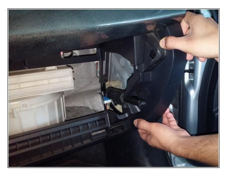
Carefully remove the plastic trim by pulling outwards.
