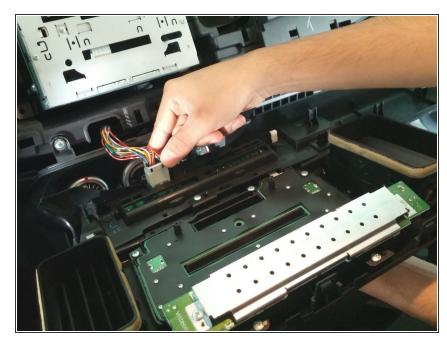
i Optional: If you choose, you can remove the harness shown. (See directions on Step 12 for removing a harness clip.) Otherwise you can simply rest the fixture on top of the shift knob.
