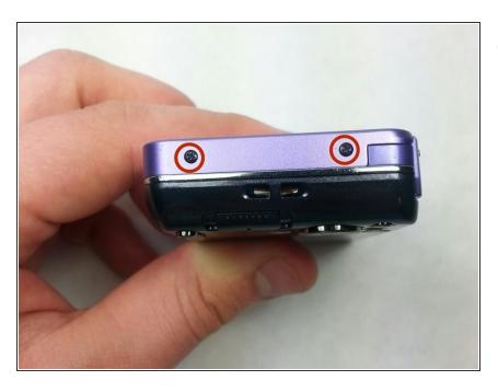
Turn the camera sideways so the left side is fashing upwards, remove the two Phillips head, 2.93 mm screws.
