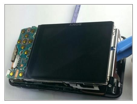
Remove the LCD screen from the side opppsite the battery terminals.
