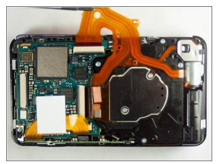
This is what the camera should look like after 2 cords and the screen have been removed. The lens cord is being held to the side for a clearer view.
