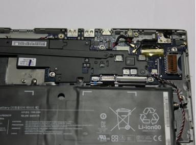
Remove the metal cover above the charging port module by pulling up and moving it slightly left.
