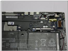
Unscrew the 3.4 mm screw holding down the charging port module using a Phillips #00 screwdriver.
