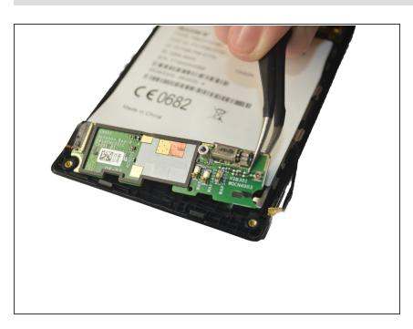
Finally, remove the keyboard module by pulling it up with the tweezers from right to left.
