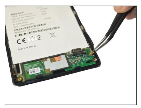
By using the tweezers, unclip the cable at the bottom right by pulling it up.
