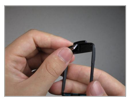
When the speaker is loose, gently lift the speaker out of the panel.
