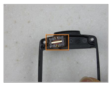
Locate the speaker on the back of the removed panel.
