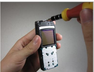
Using a T6 Torx Screwdriver, unscrew and remove the six screws shown in the picture.
