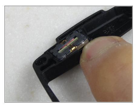
Use nails to gently lift the speaker up; speaker may be slightly glued to the panel.
