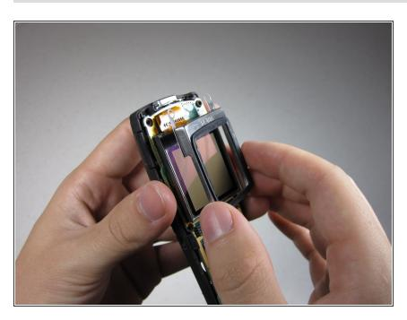
Remove the LCD screen frame.
