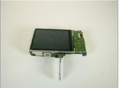
Remove the main back piece. It should easily lift off.
