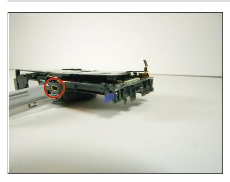
Use the spudger and slide the plastic case over the mini USB port.
