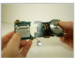
Now with one hand located on the plastic skeleton and the other on the motherboard pull the motherboard to the left to disconnect the last ribbon.
