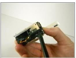
After the screen is off, work the spudger under three clips to remove the metal plate.
