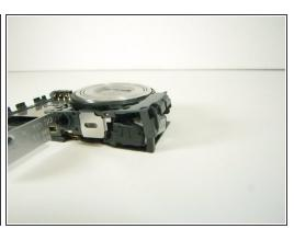
Use the spudger and disengage the black plastic clip located on the bottom right of the camera facing the lens.
