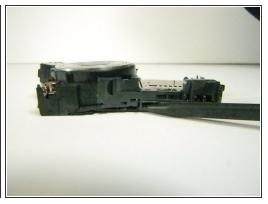
• Use the spudger to disengage the plastic clip on the top of the camera.
