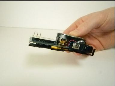
• Use tweezers to disconnect the ribbon located under the motherboard near the bottom of the camera.
