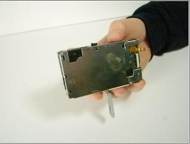
Slide the right side of the LCD screen clockwise, which will push it off the camera. The rest of the screen should come off with it with ease.
