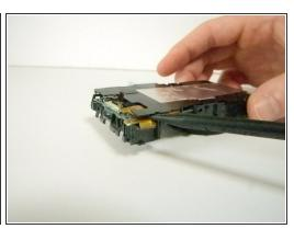
• Flip the camera over, facing the bottom of the camera towards you. Then use the spudger to detach the plastic clip on the right, near where the LCD control board was.
