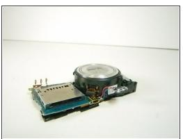
Use the spudger and seperate each end of the metal piece. Once the speaker is free you can lift off the plastic frame.
