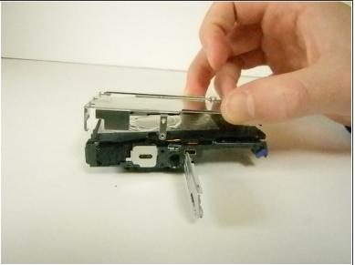
After the clips are disengaged, lift off the metal cover.
