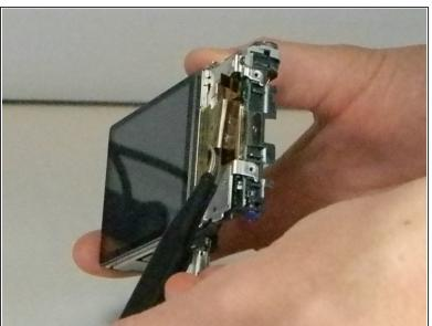
Use tweezers to remove the ribbon that is connected from the LCD screen to the camera by pulling the part that is folded under, out.
