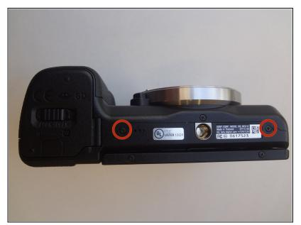
Remove the two 3.5mm Phillips #00 screws that hold the back case - located on the bottom of the camera.
