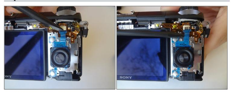
• Pry out the ribbon cable by carefully pushing on its side tabs with a spudger.
