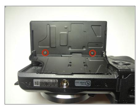
Remove the two 1.0 mm Phillips #00 screws from back of the LCD screen.
