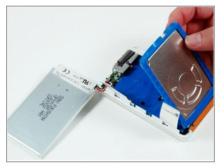
Lift up the end of the hard drive near the Firewire port to allow easy access to the battery connector.
