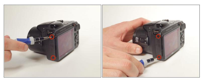
Remove two 5 mm Phillips #000 screws near the audio/video inputs on the opposite side near the flash component.
