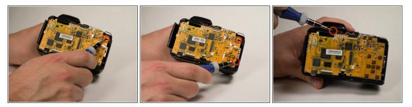
• Remove three 5 mm Phillips #000 screws bordering the motherboard.
