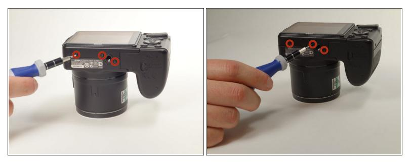
• Remove three 5 mm Phillips #000 screws on the bottom end of the camera.
