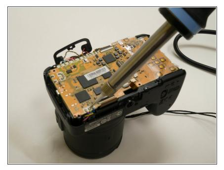
• Unsolder the wires on the bottom end of the motherboard.
