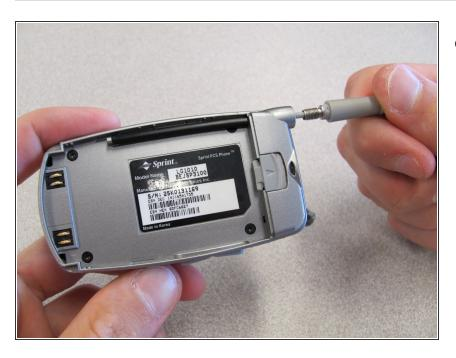
While holding cell phone firmly in one hand, unscrew and remove the antenna with the other hand.
