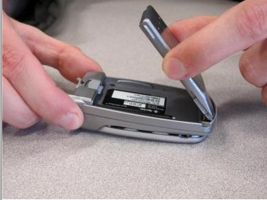
While sliding the gray tab up, lift battery up and away from the cell phone.
