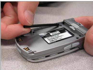
Pull the antenna housing (black tube) towards bottom of phone and remove.
